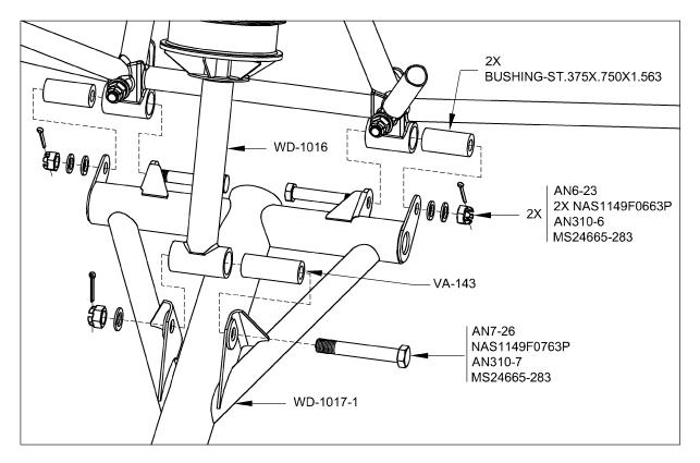
**FIGURE 2:** NOSE GEAR ATTACHMENT
